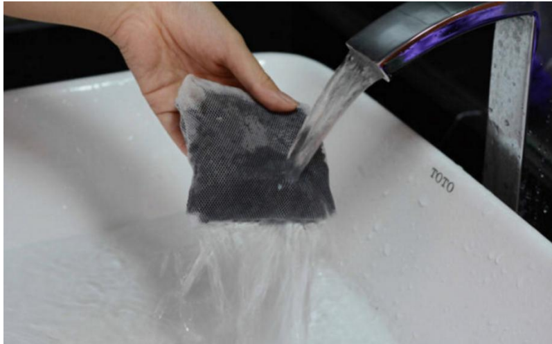
9. Rinse the activated carbon with water until no black water flows out
